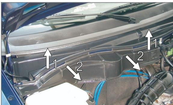
**EN** Remove the electric circuit housing
