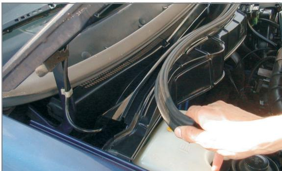
**EN** Remove the rubber seal
